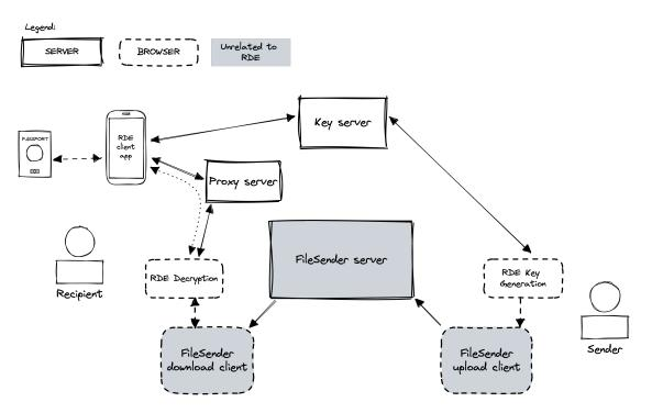
Figure 4.3: Overview of the RDE infrastructure integrated in the FileSender application.
