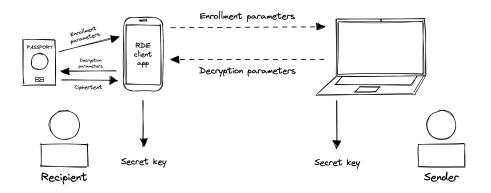
Figure 2.1: High-level overview of the basic RDE scheme.
